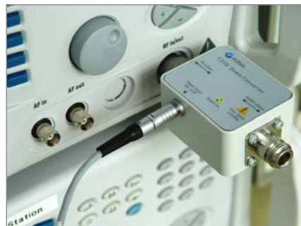
Figure 2: The 1209 Downconverter is an optional frequency extension for Bluetooth, WLAN, GPS tests and Mobile TV standards.
